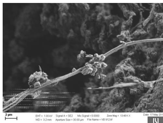
Figure 4. SEM analysis of mixed sample (VB + chrysotile)
